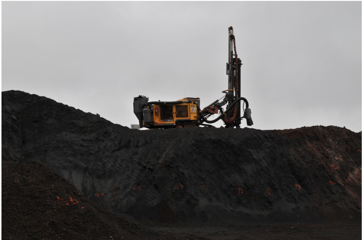
Above: Blast hole drilling rig above exposed dark hematite ore face at the James Pit.
